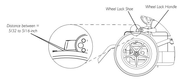
FIGURE 13.1 Installing/Adjusting/Using the Wheel Locks
